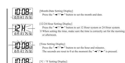
**②**Press the "TIME SET" to return to the normal time display after adjusting the settings.
